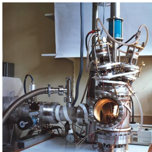
Tri arc pulling furnace for Czochralski growth experiments.
