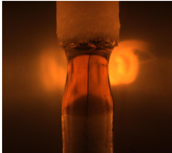
Growth of a \text{Li}_6\text{Eu}(\text{BO}_3)_3 single crystal by the optical floating zone method ( R. Belhoucif/M. Velazquez – ICMCB ).
