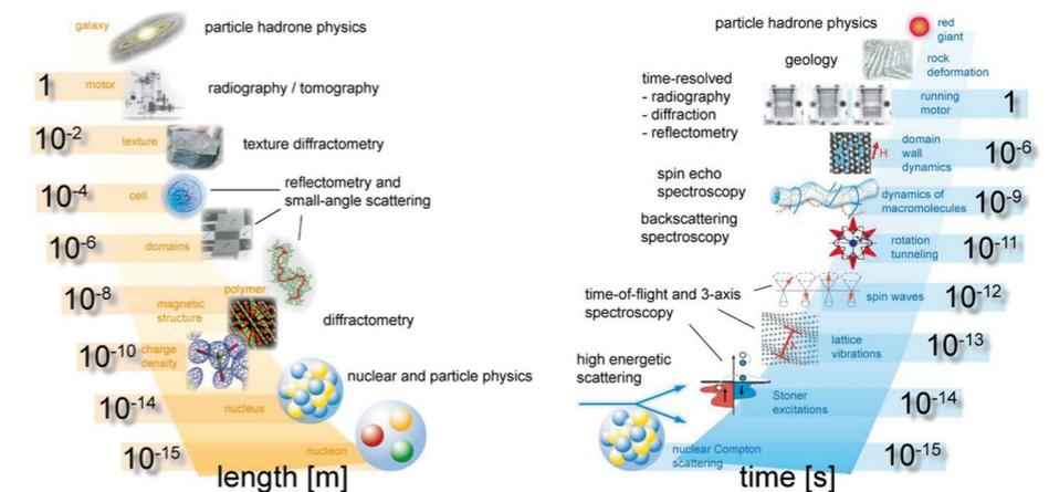
Figure 2. Length and time scales of neutron techniques
