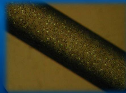
Glass capillary tube containing white protein crystalline precipitate in brass sample holder
