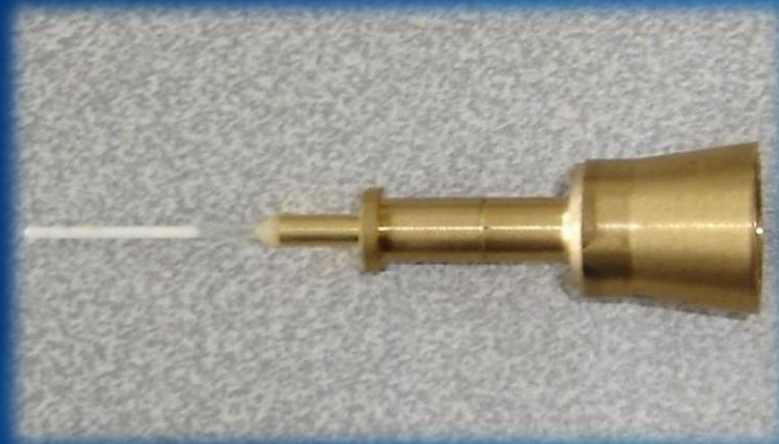
Glass capillary tube containing white protein crystalline precipitate in brass sample holder
